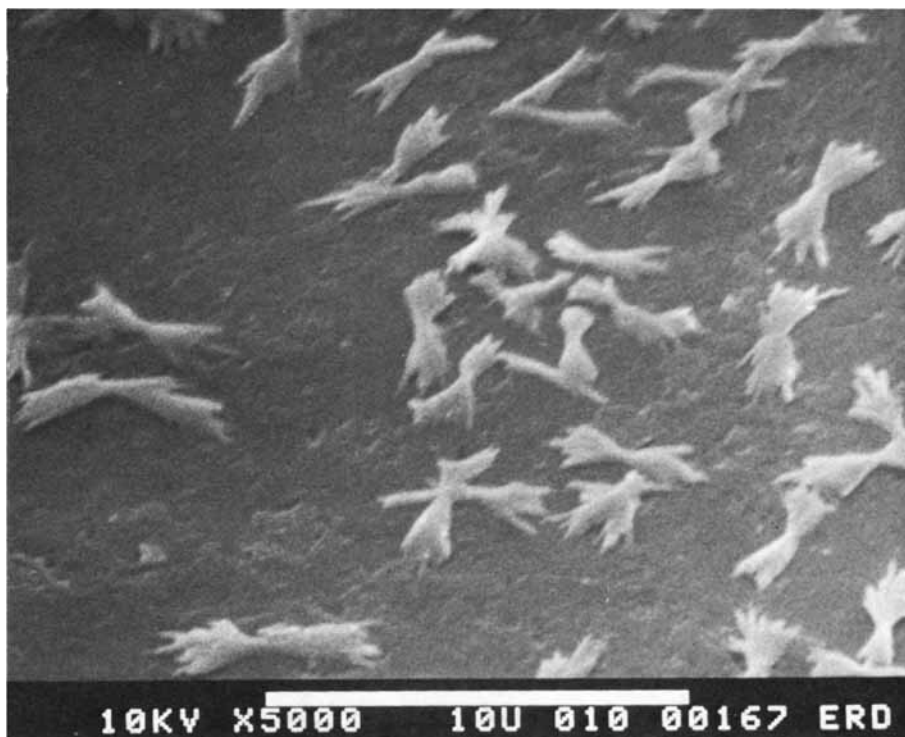
Fig. 3. Scanning electron micrograph of the partially hydrolyzed cellulose chloral hemiacetal film. The featured platelets probably represent unevenly hydrolyzed domains.
